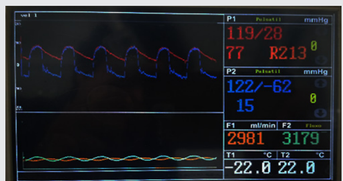
Figure 3. In the wave morphology comparison produced by the PhysioPump pumping chamber with the physiology description (taken from Guyton, Textbook of Medical Physiology, 1996).
