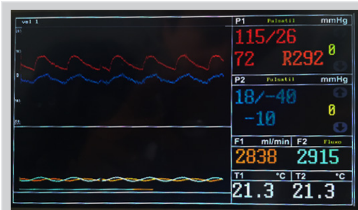
Figure 2. The red line is the pressure variation record generated by the PhysioPump pulse, the values in red 115/26 and 72 refer to systolic, diastolic pressures, and arterial line average values. Similarly, the line and values in blue, refer to the circuit venous line. The F1 and F2 captions on screen refer to arterial and venous flows, T1 and T2 are the temperature values for arterial and venous line. The R292 caption addressed a development functionality.
